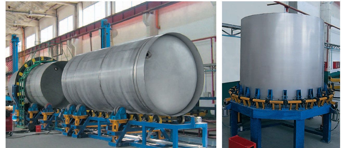
Tank assembly and welding line
