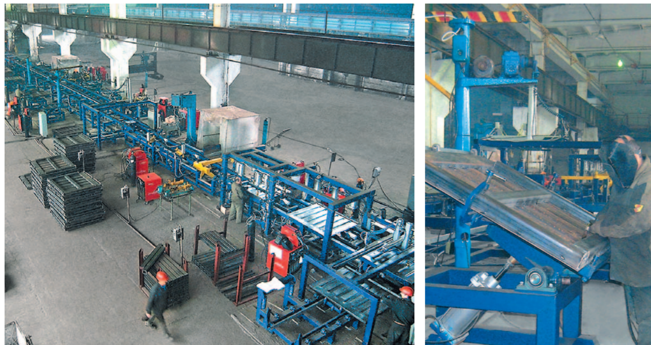
Integrated mechanized line for assembly and welding of gondola car hatch covers
