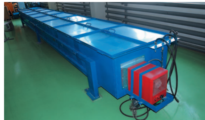
Bath for pipes testing
