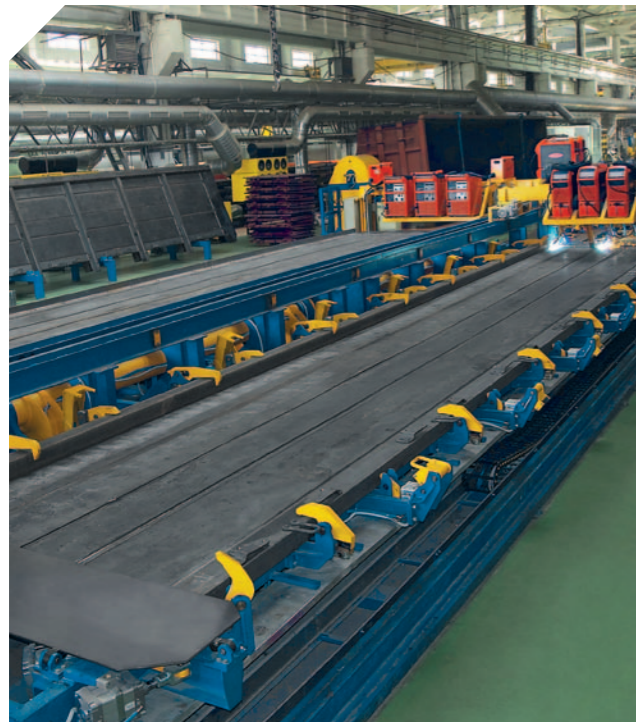
Gondola car side walls assembly and welding line
