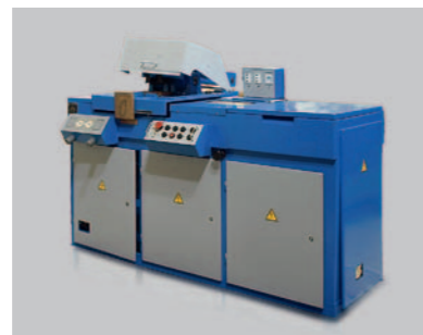
Resistance welding plant for rods
