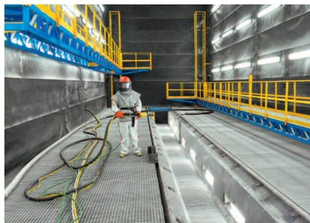
Shotblasting chamber for cars
