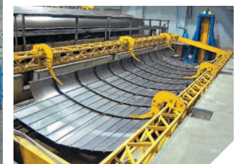
Rotator for roof welding
