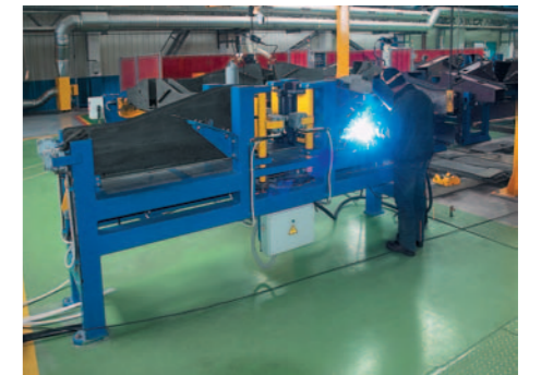
Intermediate beams assembly and welding line
