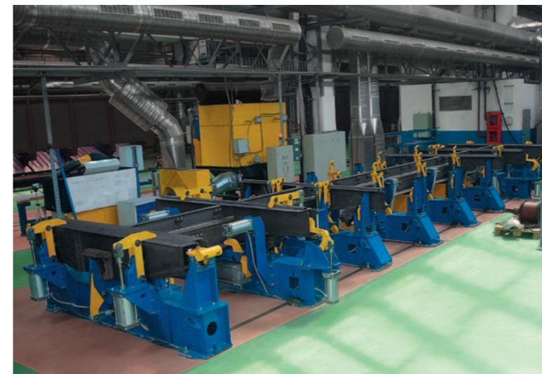
Gondola car underframes assembly and welding stand
