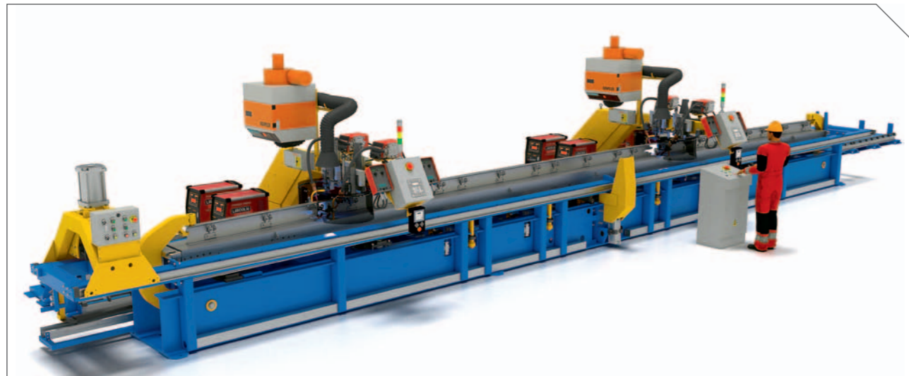
STAND FOR AUTOMATIC WELDING OF CENTER SILL WITH I-BEAM
