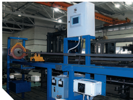
Pipes magnetic particle inspection stand
