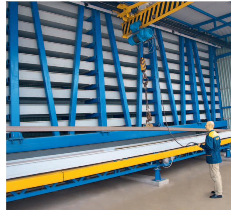
Automated storage system for section material
