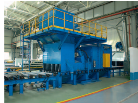
Shotblasting chamber for cleaning of metal-roll
