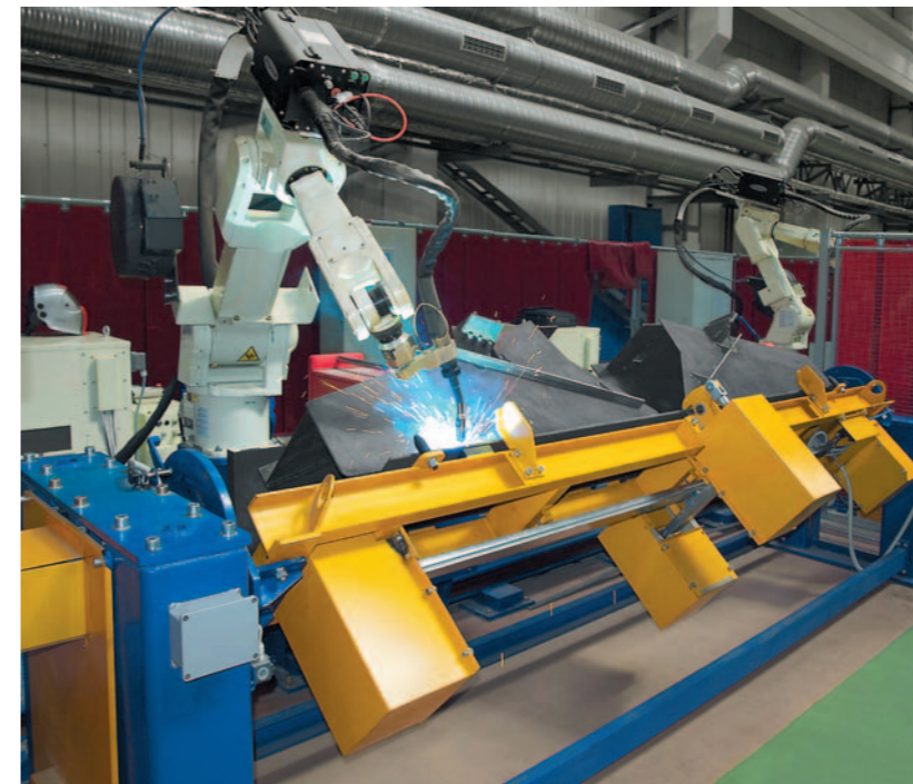
Gondola car underframes assembly and welding stand
