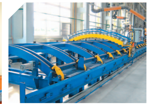
Boxcar roof assembly and welding stand
