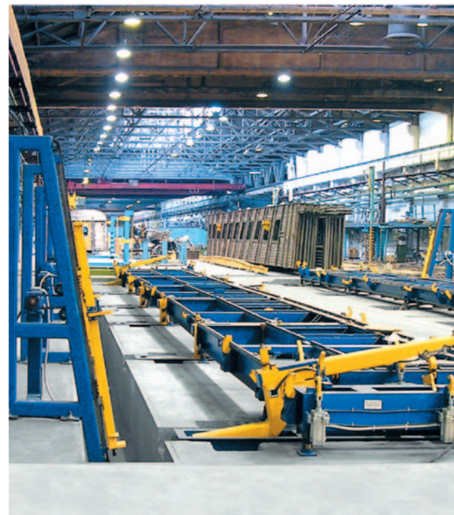
Jig-rotator for passenger car side walls assembly and welding
