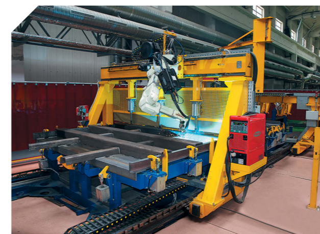
Robotic welding of the end wall posts
