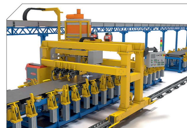
Gantry for automatic tack welding of channel bars
