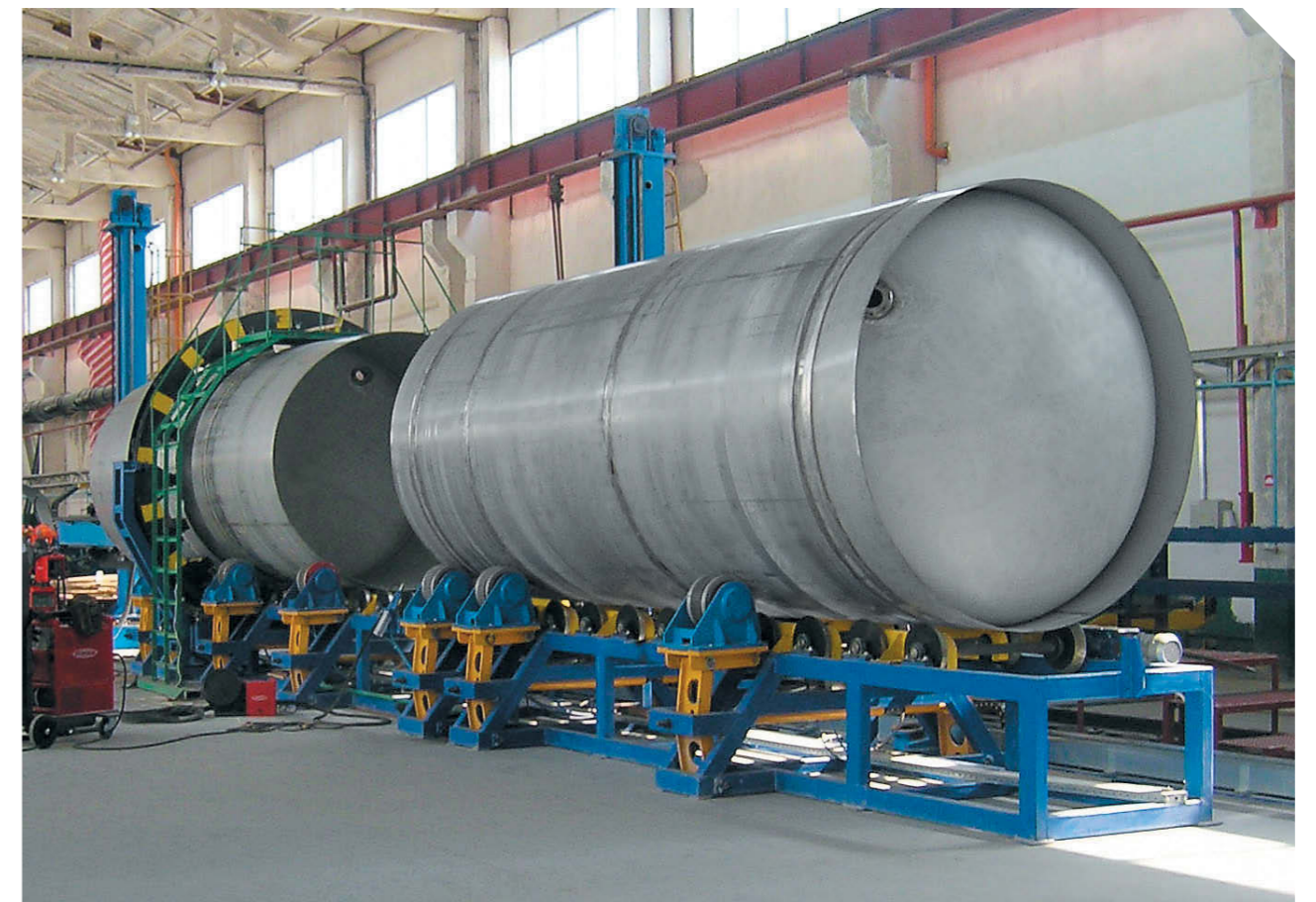
Line for assembly nad automatic welding of vessels
