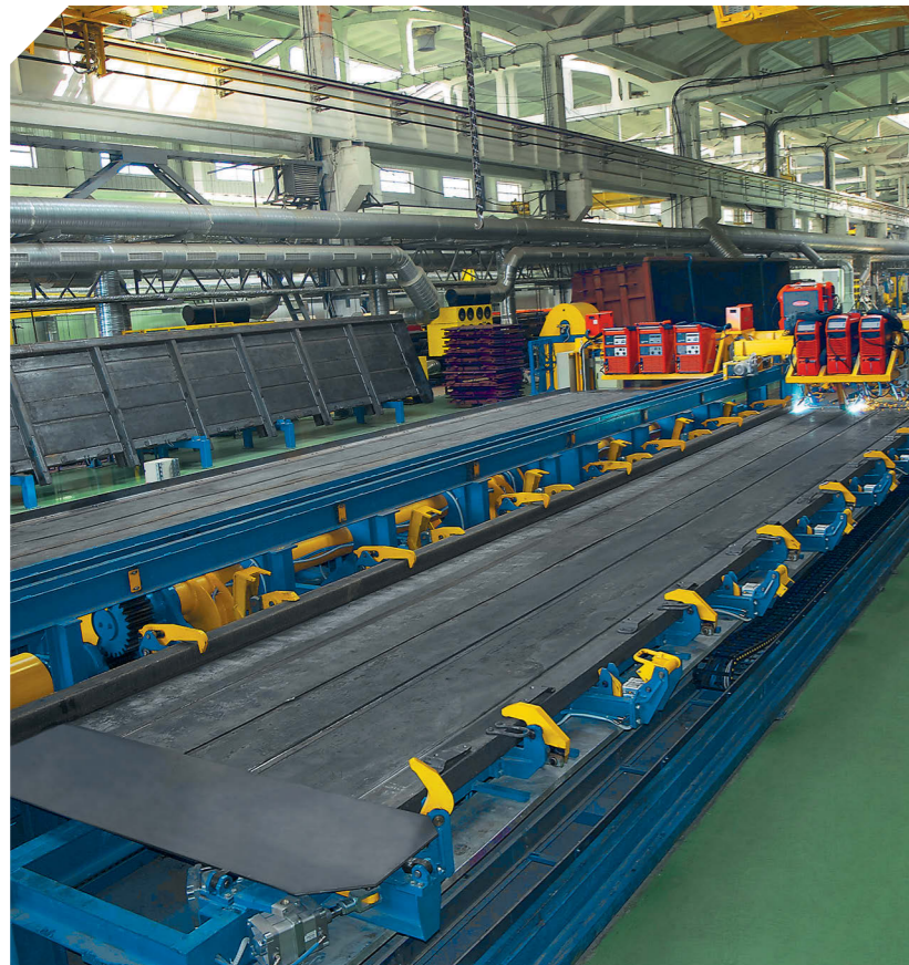
Automated center for welding of gondola car side walls
