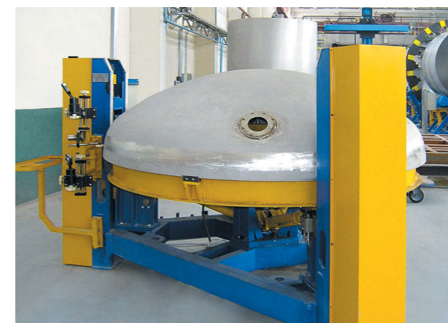
Stand for assembly, welding of vessel heads and skirt facing
