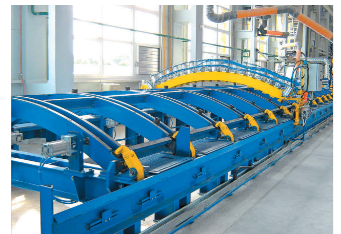
Box car roofs assembly stands
