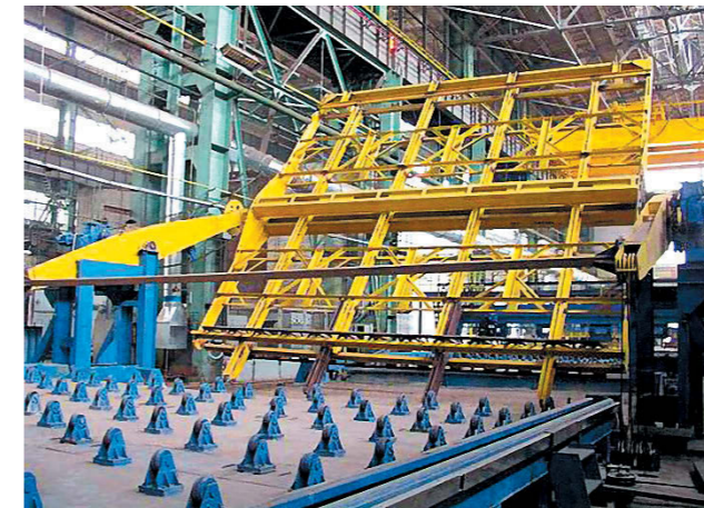
Sheets assembly and welding line
