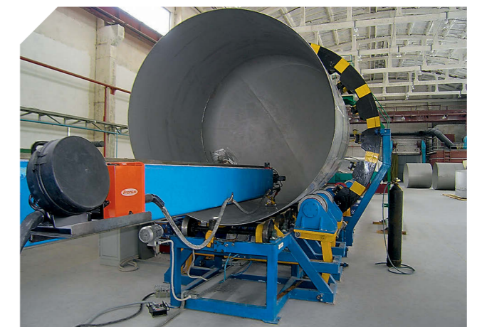
Internal seam welding
