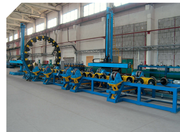
Transportation system of the line
