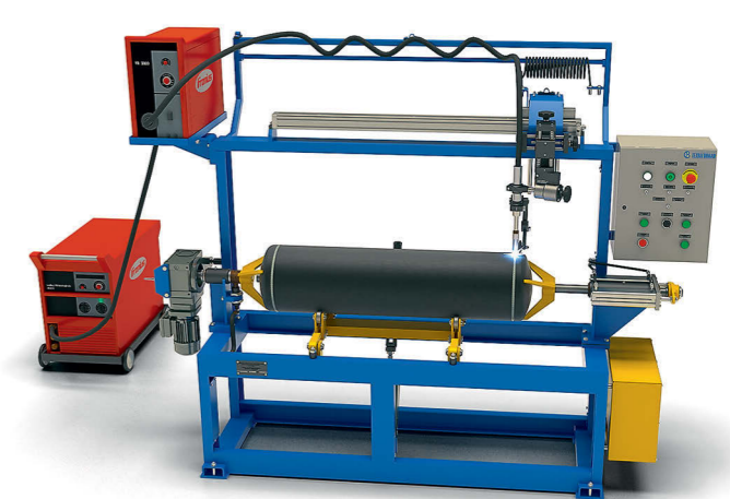
Stand for automatic welding of shell with head
