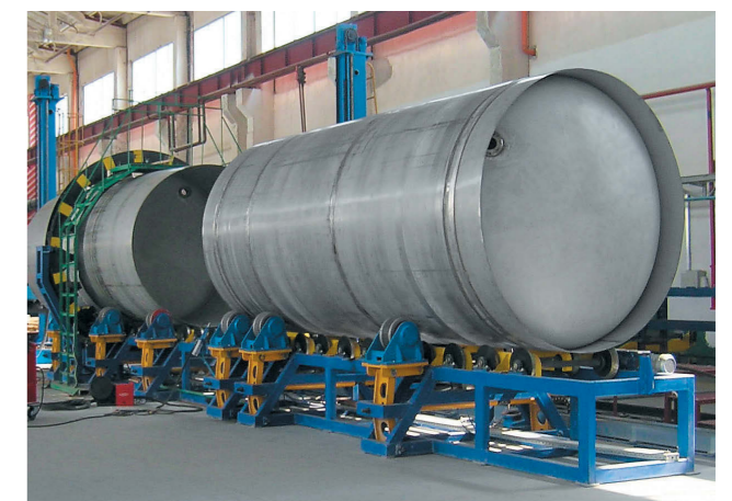
Vessel assembly and welding line
