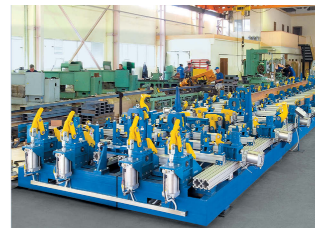
Multipurpose stand for passenger car underframes assembly
