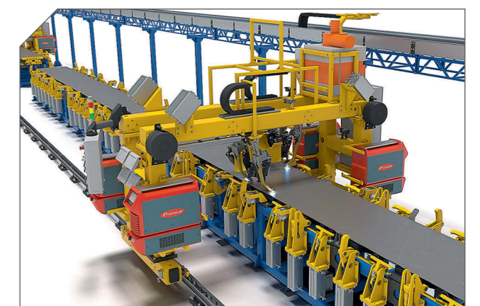
Gantry for automatic welding of longitudinal seams
