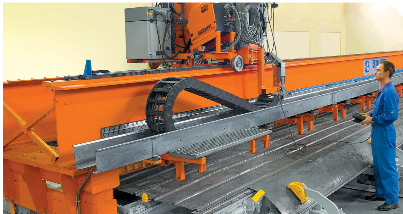
Multipurpose stand for assembly and welding of passenger cars roof sheathing
