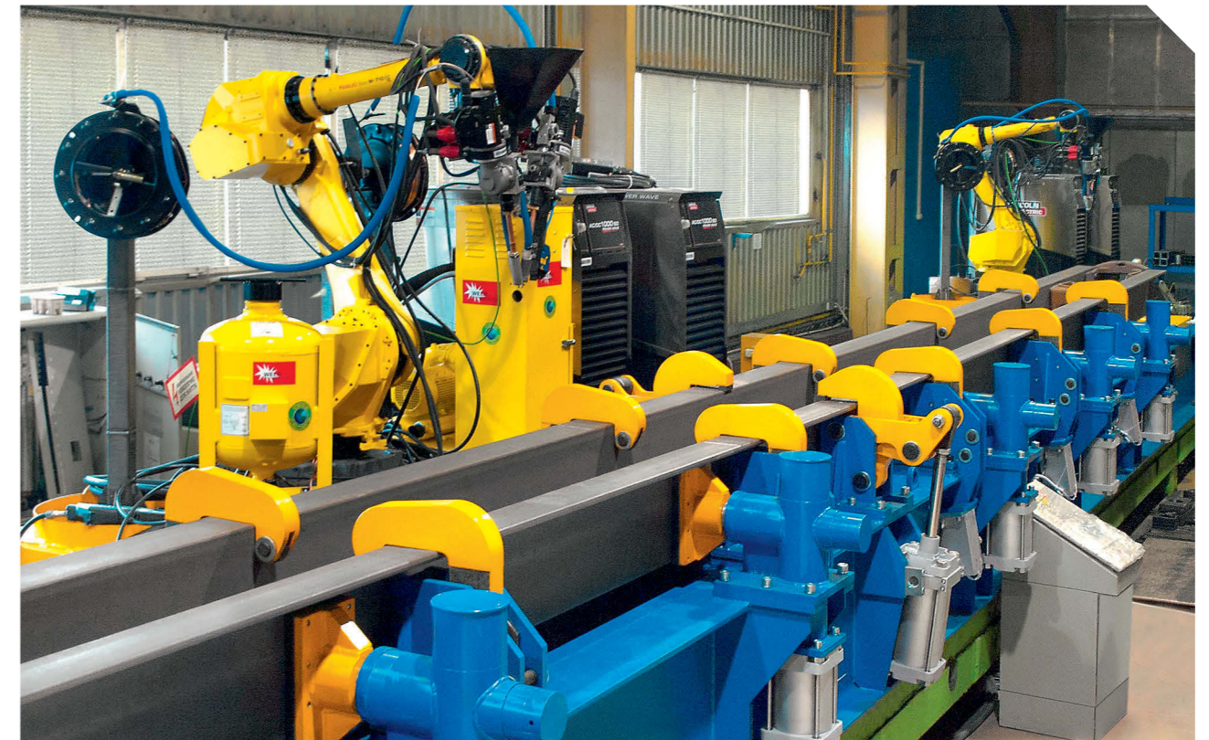
Robotic system for longitudinal seams welding
