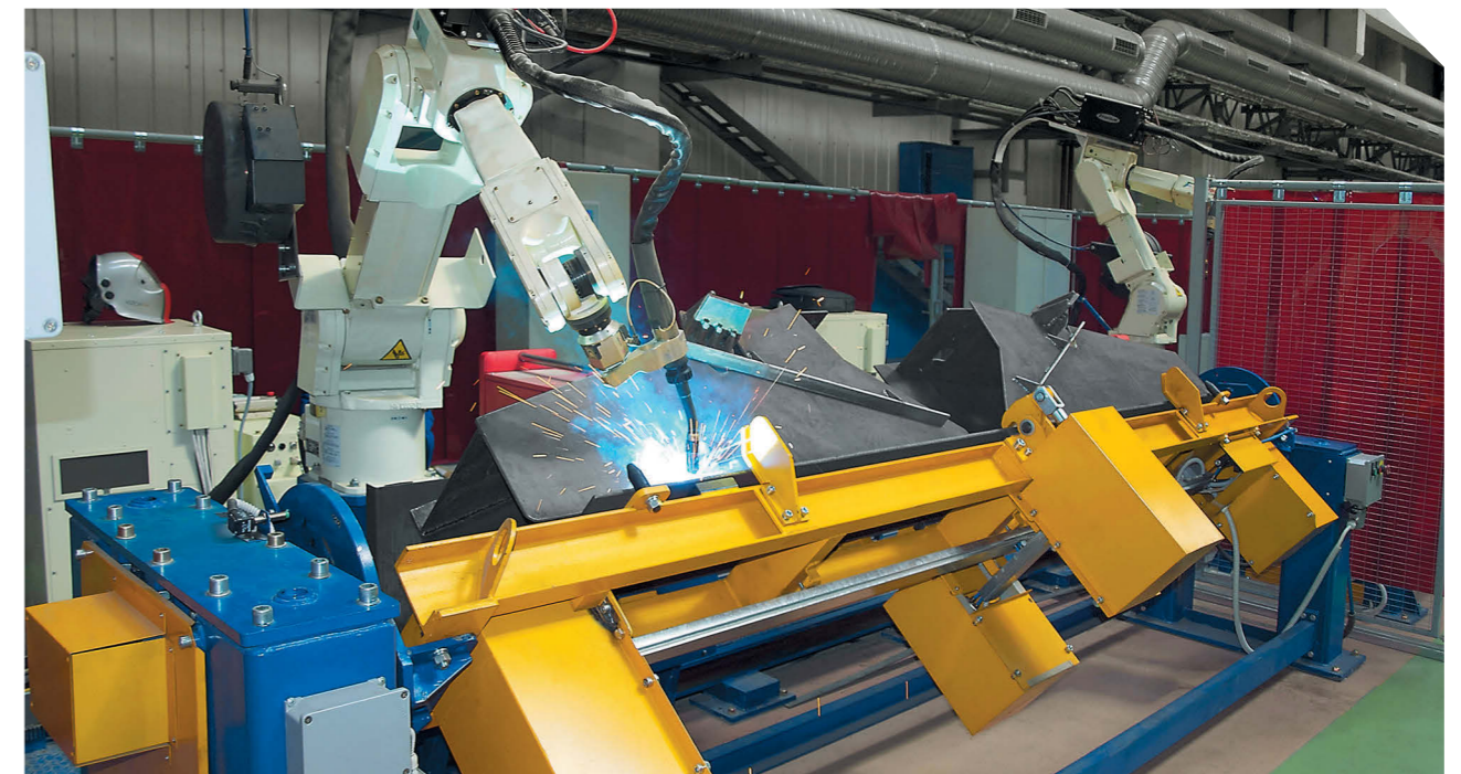
Robotic center for welding of freight cars cross bearers
