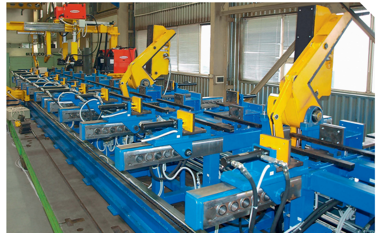
Multipurpose line for assembly and automatic welding of girders
