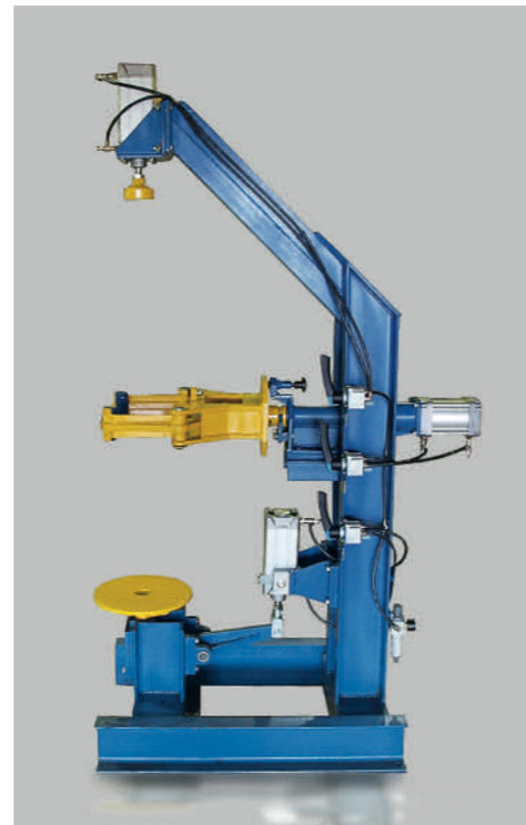
Head-to-shell assembly stand
