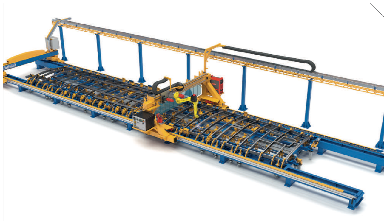
Robotic center for tram roof welding
