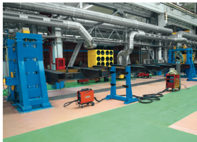
Rotator with vertical lift, load carrying capacity 15 t
