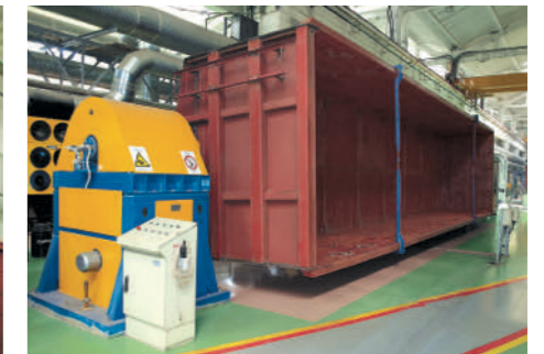
Rotator for body welding
