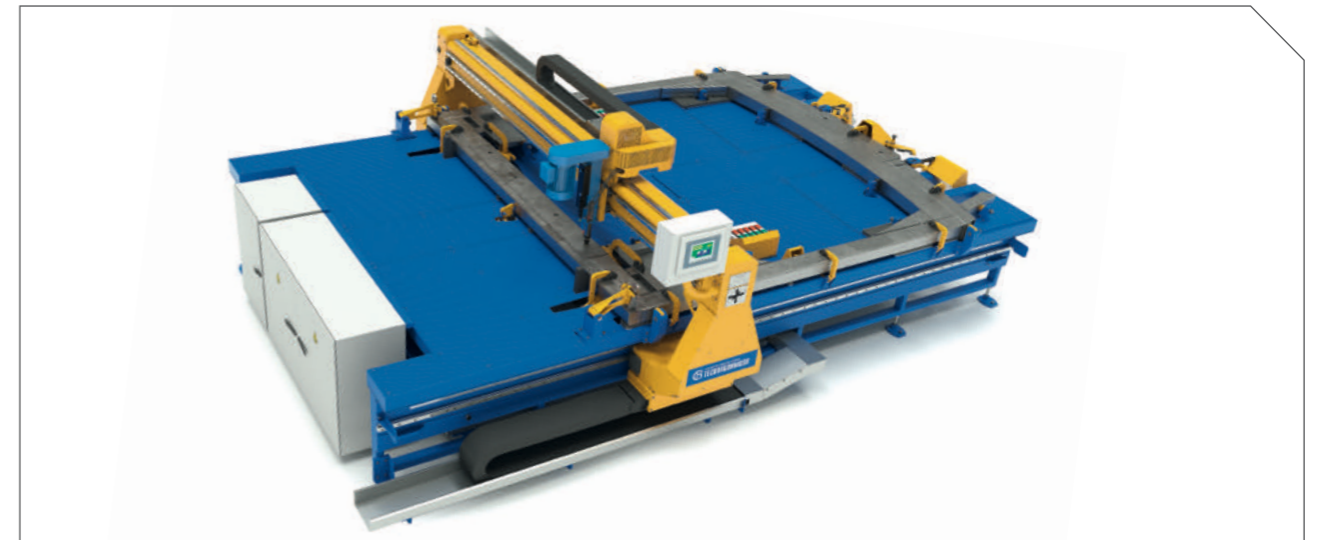
Tram sections joint frames welding and drilling stand
