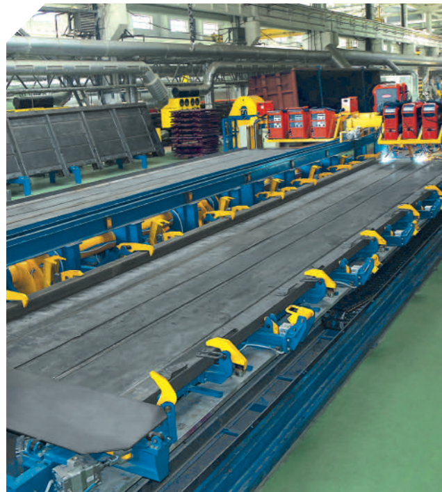
Gondola car side walls assembly and welding line
