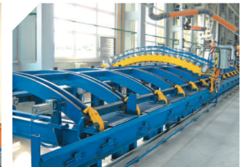
Boxcar roof assembly and welding stand
