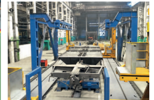
Multipurpose stand for hopper cars bodies assembly
