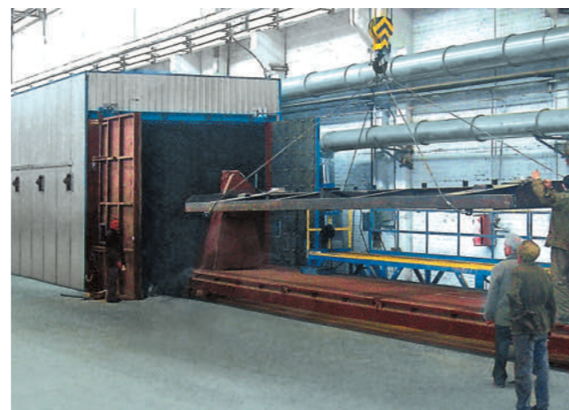
Shotblasting chamber for car underframes
