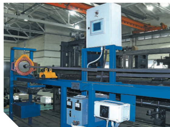
Pipes magnetic particle inspection stand
