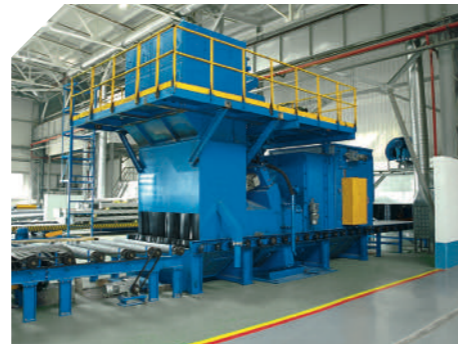
Shotblasting chamber for cleaning of metal-roll
