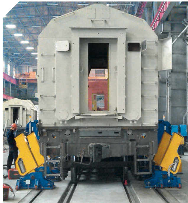
Mobile jacks for locomotives
