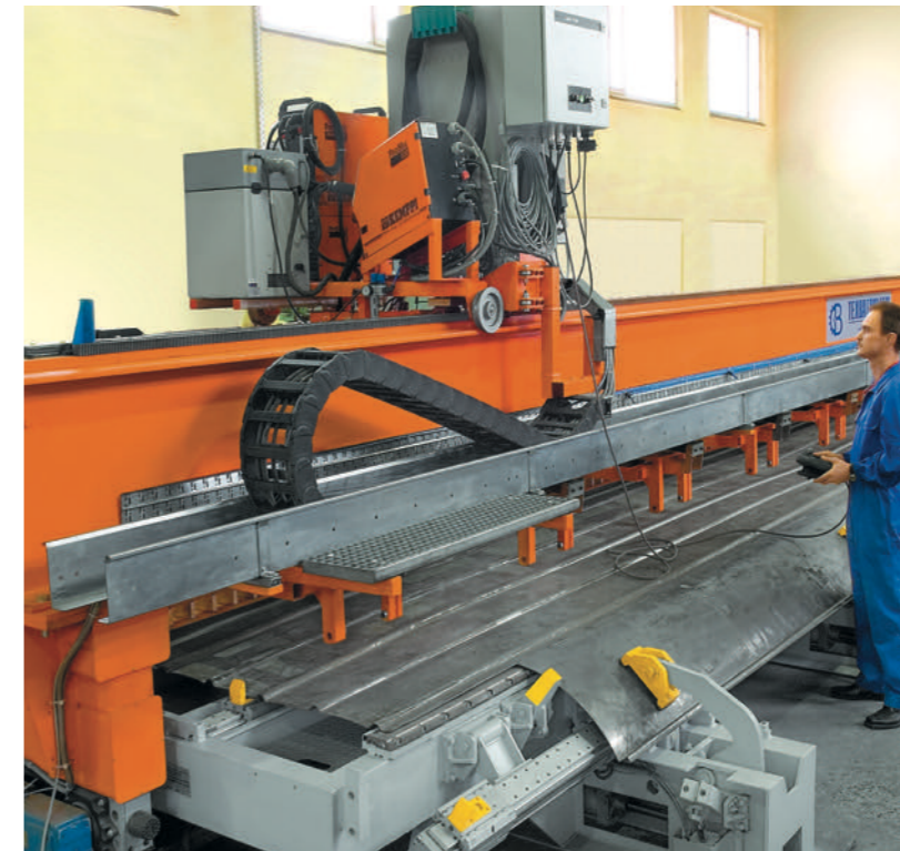
Assembly and welding stand for passenger car roof sheathing
