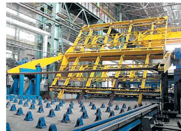
Sheet assembly and welding line
