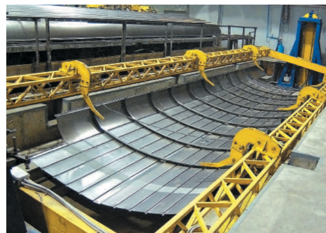
Rotator with vertical lift for passenger cars roofs welding
