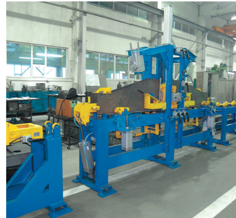
Bolsters assembly and welding line
