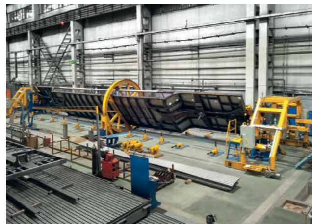
Rotator stand for double-deck passenger cars underframes welding, load carrying capacity 10 t
