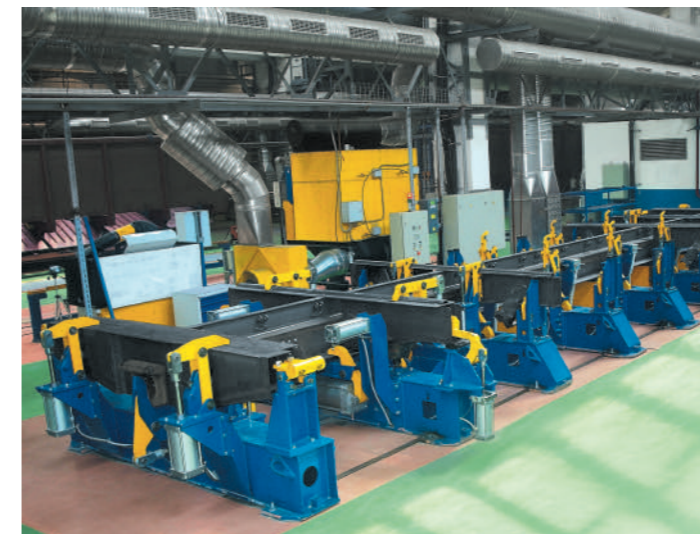
Gondola car underframes assembly and welding stand
