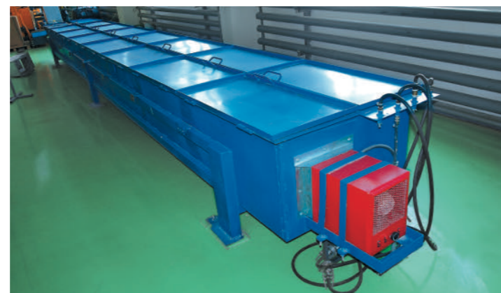
Bath for pipes testing
