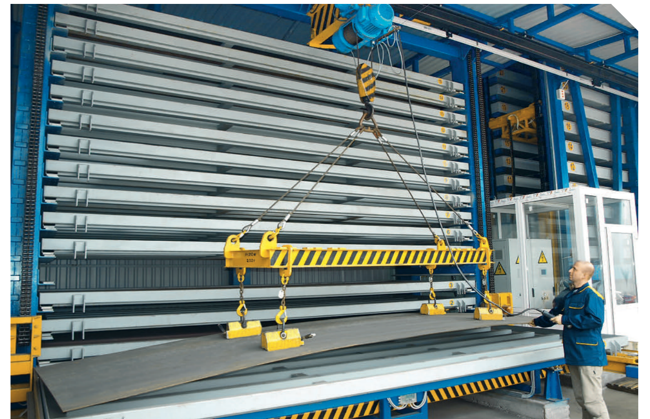
Automated storage system for sheet products
