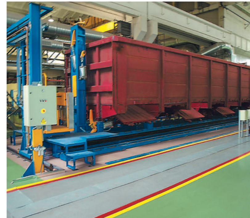
Gondola car body assembly and welding stand
