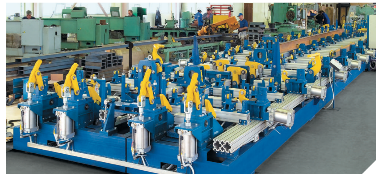
Multipurpose jig for assembly and welding of passenger car underframes
