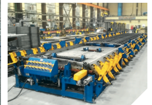
Multipurpose stand for metro coach roof assembly
