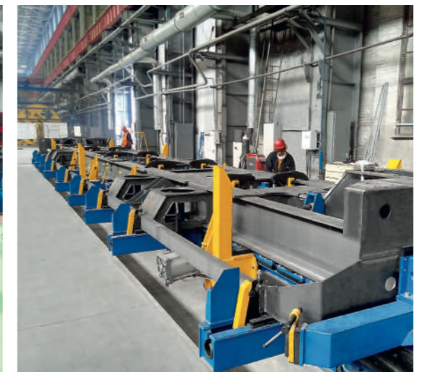
Locomotive frames assembly
