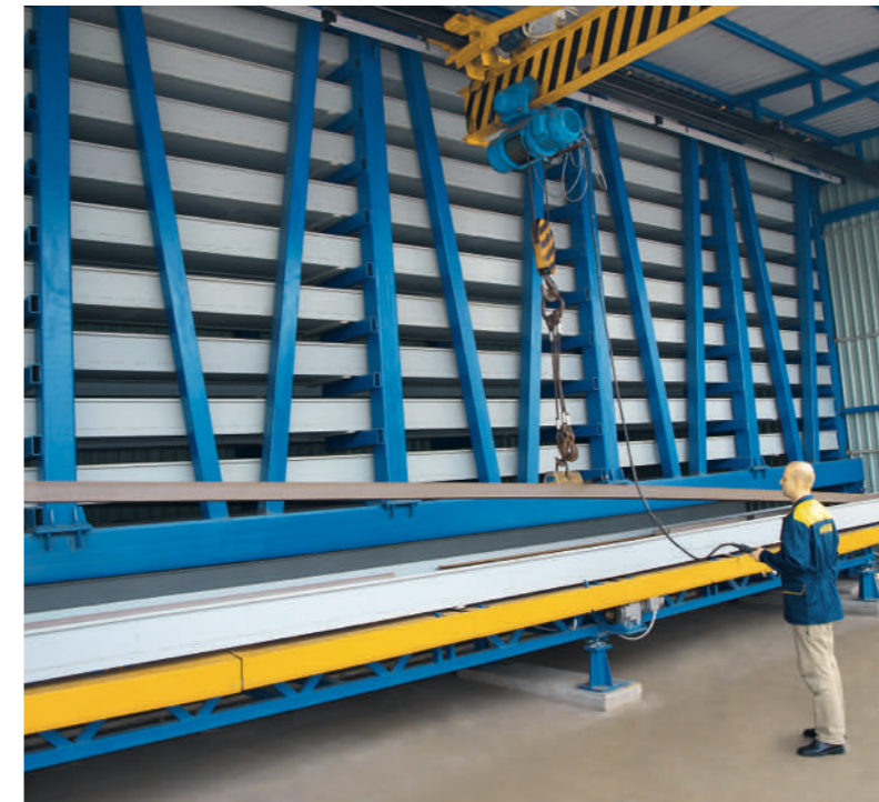
Automated storage system for section material
