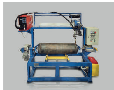
Stand for automatic head-to-shell welding
