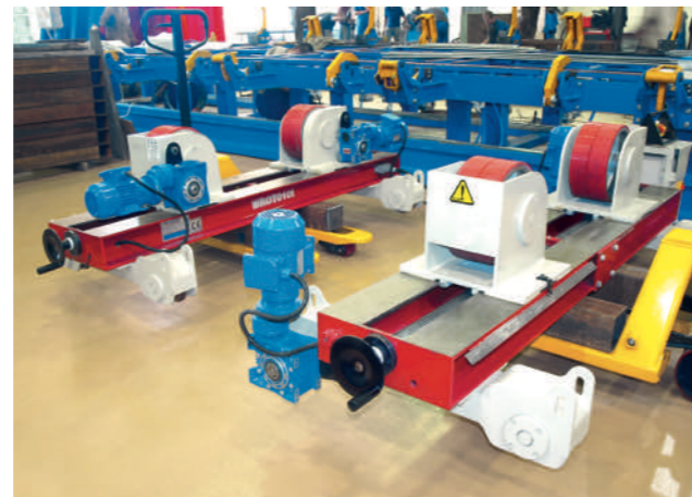
Carrying rollers with different load capacity
