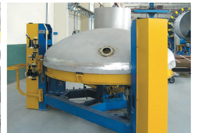
Tank head assembly and welding, edges trimming stand
