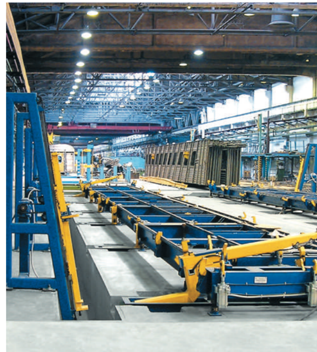
Jig-rotator for passenger car side walls assembly and welding
