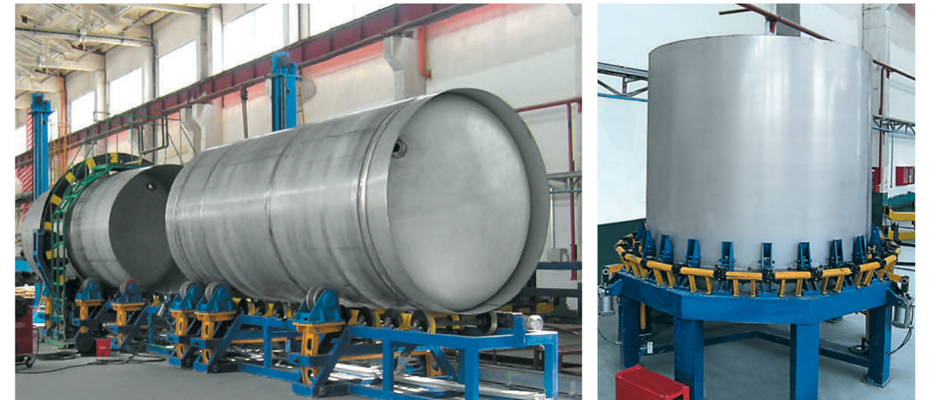
Tank assembly and welding line
