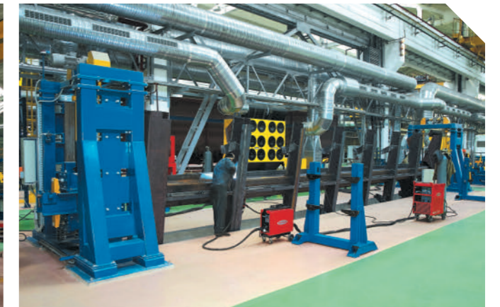
Rotator for underframe welding
