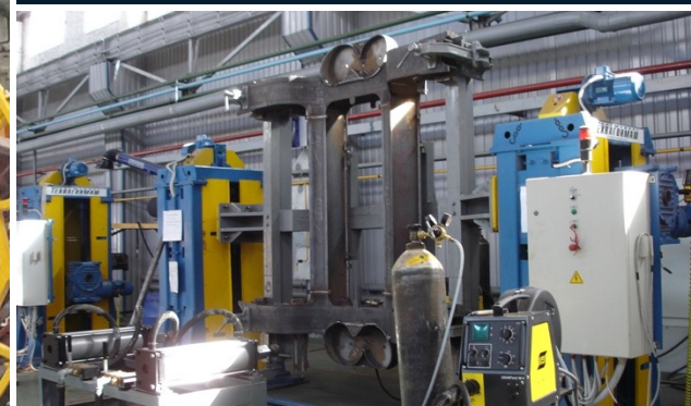
Positioner for bogie frame
