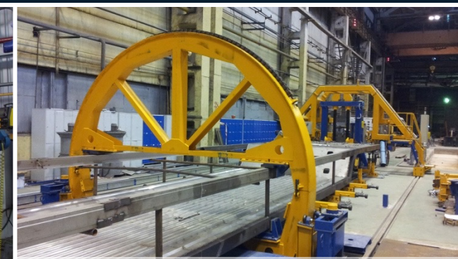
Positioner for frames of double-deck carriages
