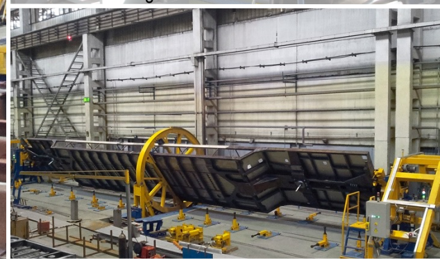
Positioner for frames of double-deck carriages
