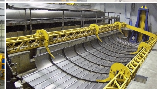
Rotator for car roof covering sections
