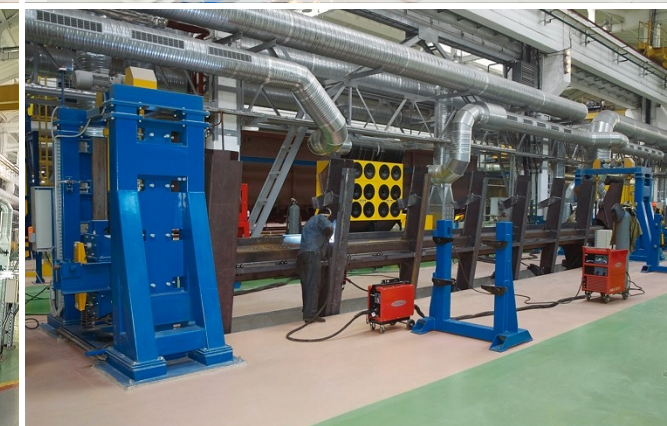
10 t welding rotator
