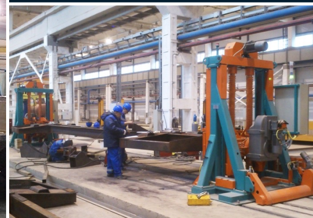
15 t welding rotator
