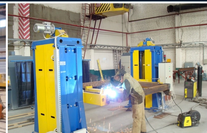
4 t welding rotator
