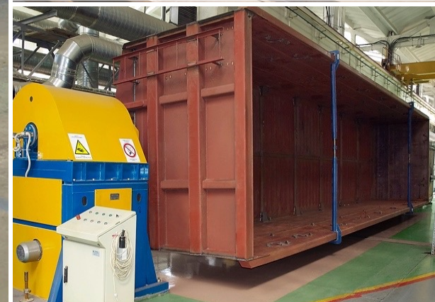
Welding rotator for gondola car body
